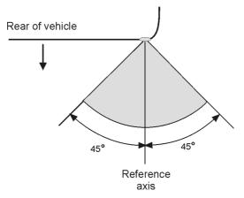
also 15° up and 15° down if lamp height is 750mm or higher or 5° down if lamp height is less than 750mm.
