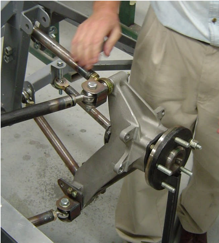
Figure LS7 Heim Joints used in a suspension application
