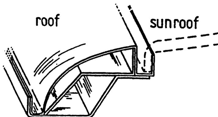
Figure LH7 Cant Rails and Sun roof Frame
