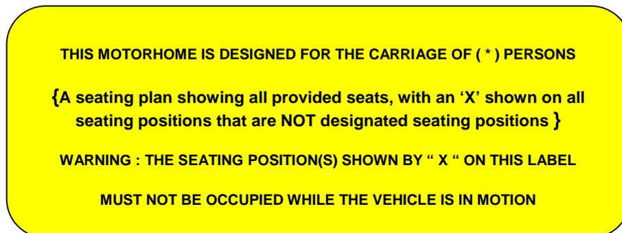
**Figure LH16 Warning Label Including Seating Plan (for seats that must not be occupied when the vehicle is being used on public roads)**
