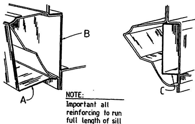
Figure LH5 Alternative Sill Details
