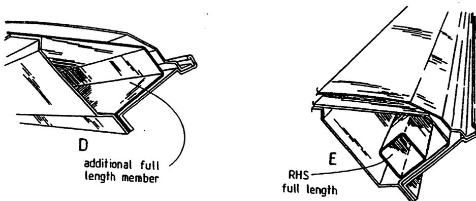
Figure LH10 Cant Rail Reinforcement Details
